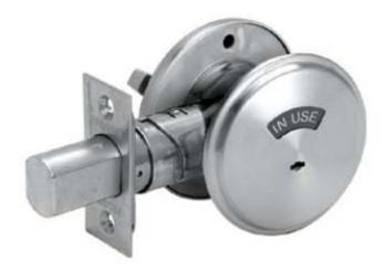
Deadbolt thrown or retracted by turn unit only. Occupancy indicator on outside (reads either "in use" or "vacant" with color coding). Bolt automatically deadlocks when fully thrown. Emergency key supplied.
